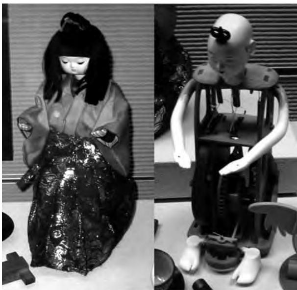
FIG. 7. Tea serving Karakuri is a doll which serves a cup of tea on its arms to a people by coming towards the front then returns to its starting position when the tea cup is put back to the arms[12].
